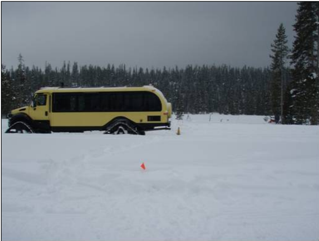
Figure 12. Purpose built International Bus with “Grip Trax” Tracks (NPS Snowcoach)
