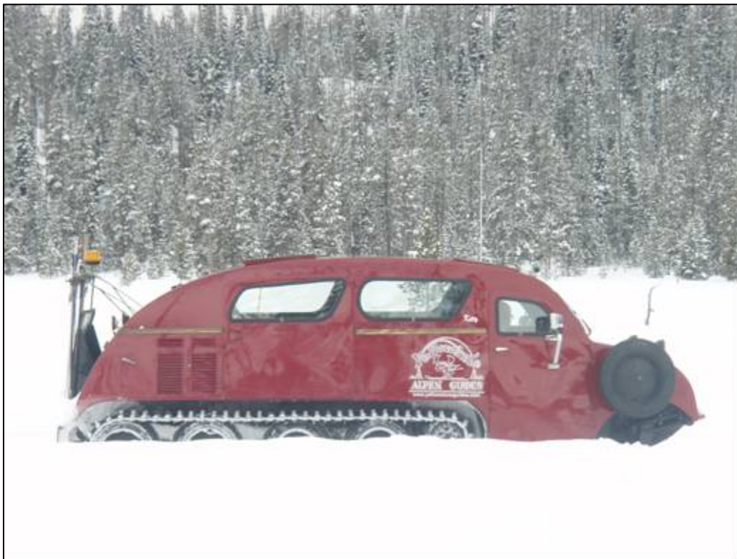
Figure 6. Purpose Built Bombardier B-12 with Skis and Tracks (Alpen Guide)
