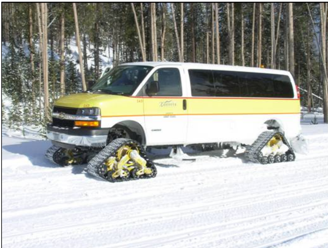
Figure 10. Customized Van with “Matracks” Tracks (Xanterra 431)
