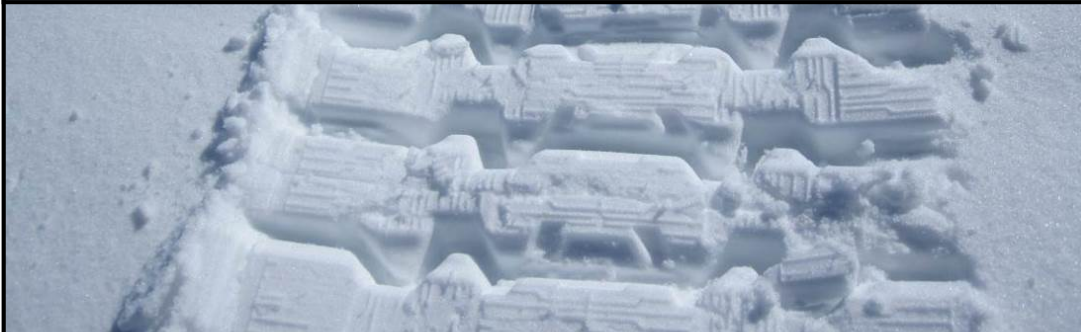
Photo J4-2: The 1" deep track lug impression left on the firm, windswept trail by the tracked Polaris RZR UTV
