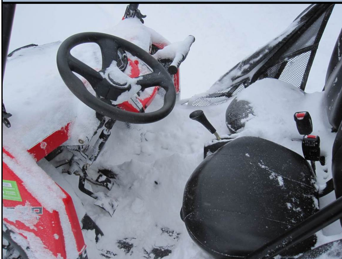
Photo J3-6: Snow deposited into cab area of the RZR during operation in uncompacted new snow
