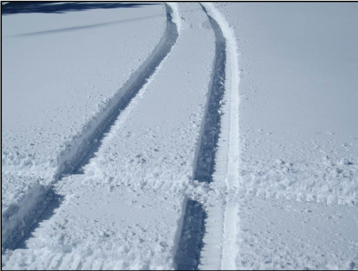
Photo J4-8: The 4" to 6" deep track impressions created by the tracked RZR when operated off- trail in deeper, softer snow
