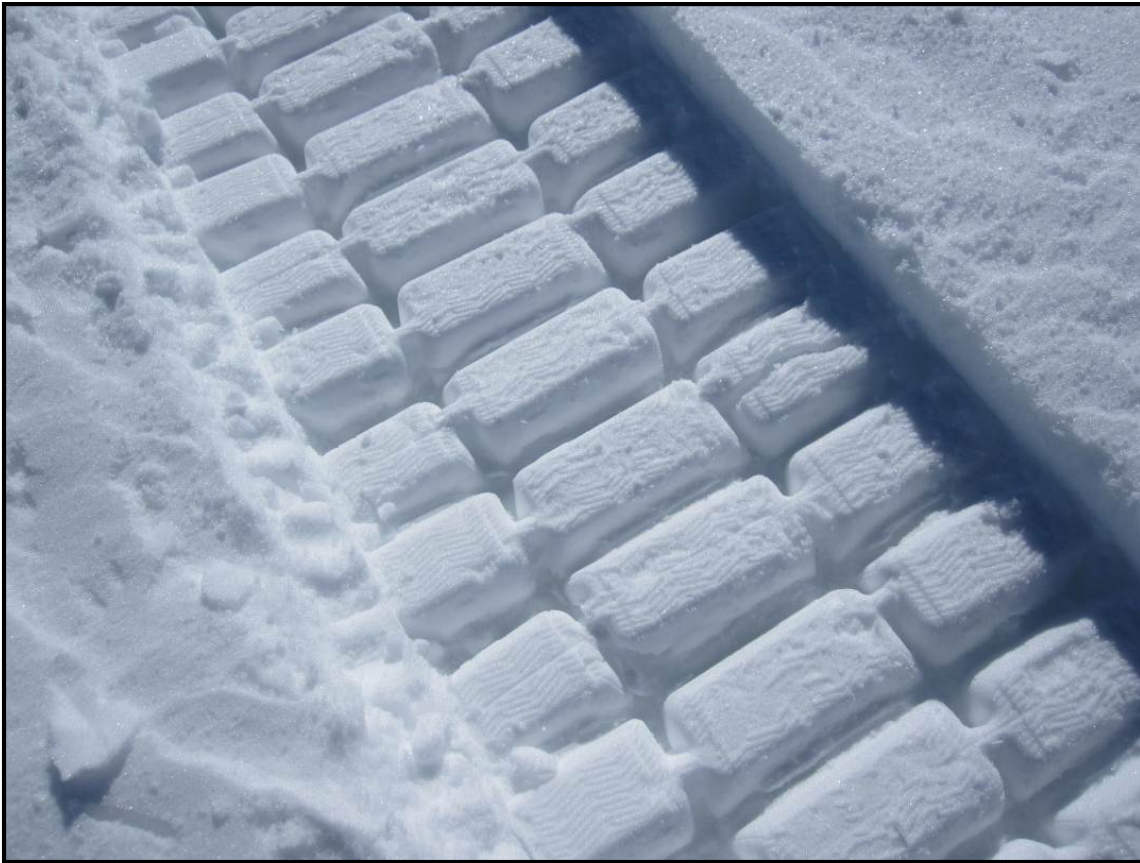
Photo J4-12: The 2''' deep track impression created by the tracked ATV when operated off- trail in firmer, windblown snow
