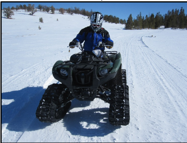
Photo 2-1: Tracked 2014 Yamaha Grizzly 700 46.5" wheeled width; 54" tracked width
