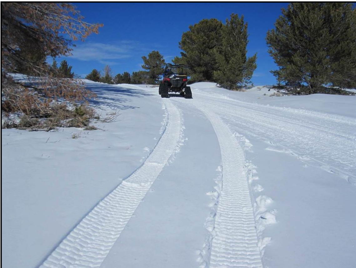
Photo J4-9: The tracked Polaris RZR transitioning from off-trail onto the CDA trail in a windswept snow area
