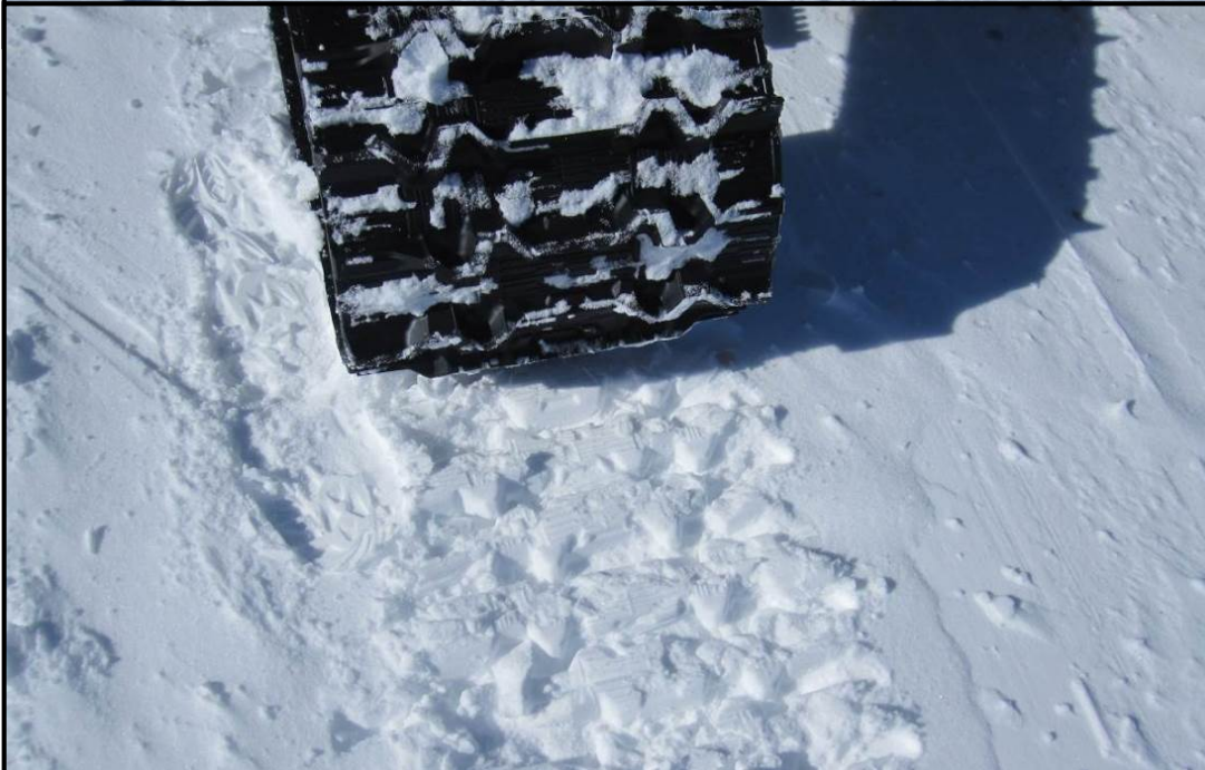
Photo J4-3: The depth of the impression left on the trail by the tracked RZR is similar to the depth of the boot impressions on the trail (to left of RZR track in photo)
