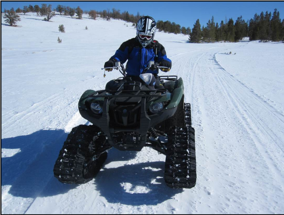
Photo J4-4: Front view of the tracked Yamaha Grizzly 700 ATV operating on the Continental Divide snowmobile trail near South Pass, Wyoming
