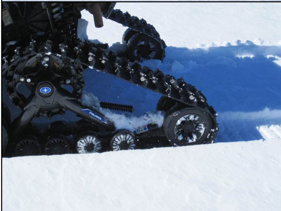
Photo J4-7: The 2" deep track impressions created by the tracked RZR when off-trail in firm, windblown snow
