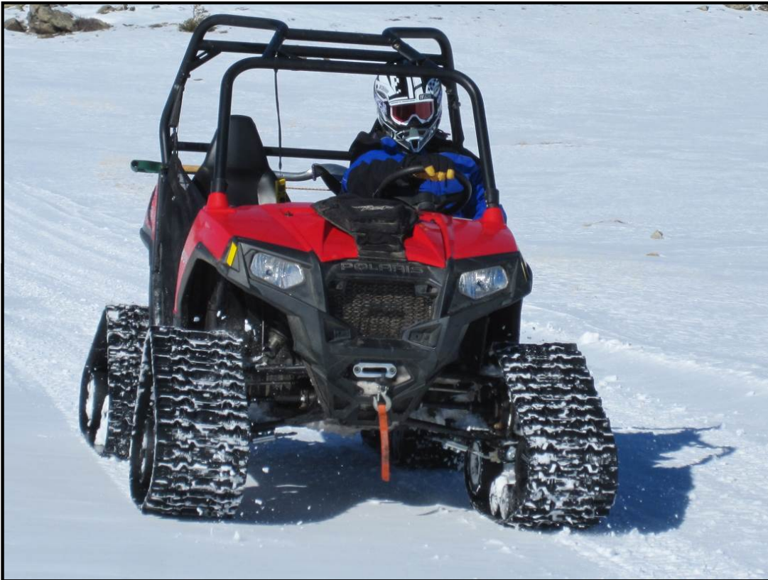
Photo J4-1: Front view of the tracked Polaris RZR 570 UTV operating on the Continental Divide snowmobile trail near South Pass, Wyoming
