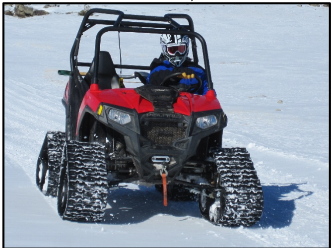
Photo 2-2: Tracked 2014 Polaris RZR 570 50" wheeled width; 61" tracked width
