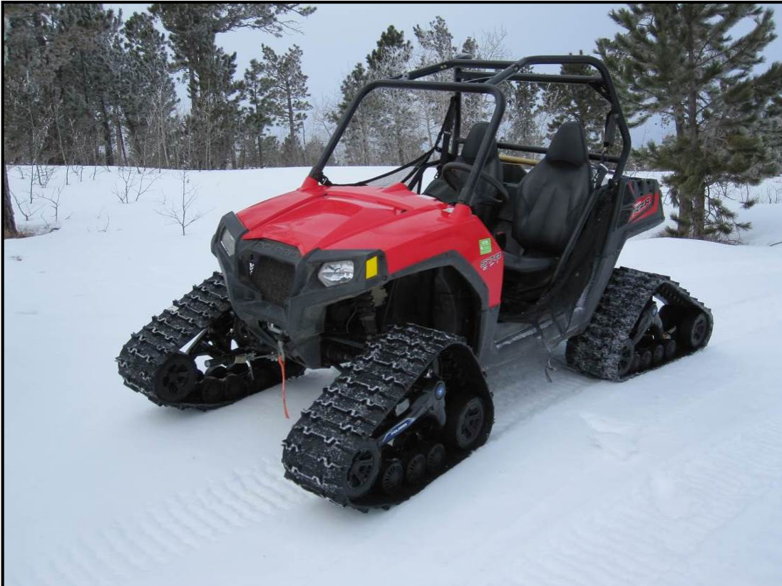
Photo J2-3: Footprints in off-trail snow (to the right of front track) are deeper than the RZR's track impressions
