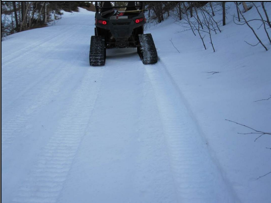
Photo J2-4: RZR track impressions with left track on-trail and right track in 2' deep uncompacted snow beside the trail
