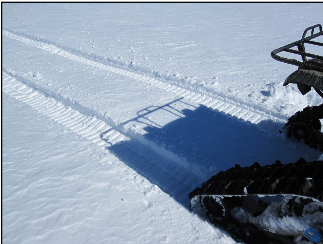
Photo J4-11: The 2" to 4" deep track impressions created by the tracked ATV when operated off- trail in deeper, softer snow
