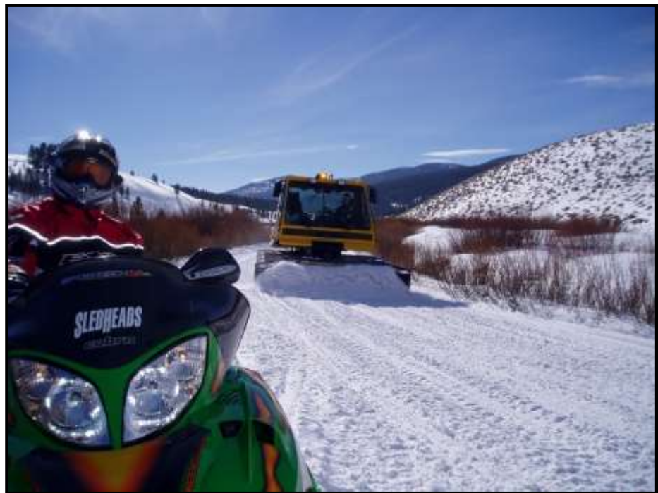
Photo 9: Example of improper front blade use on a smooth trail
