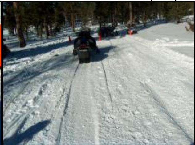
Photo 69: Impression from a fast stop
