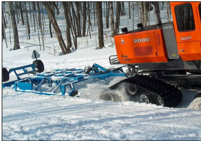
Photo 4.13 Beware of trenches dug by spinning tracks
