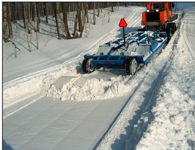
Photo 4.3 Remove back up piles! Use SMV sign.
