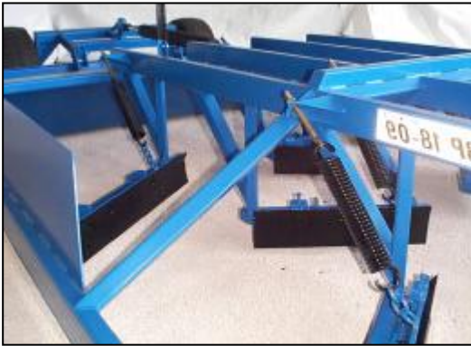
Photo 2.7 Beveled cutting blades
