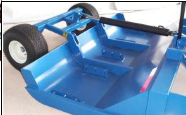
Photo 2.12 Radius lip on rear of pan
