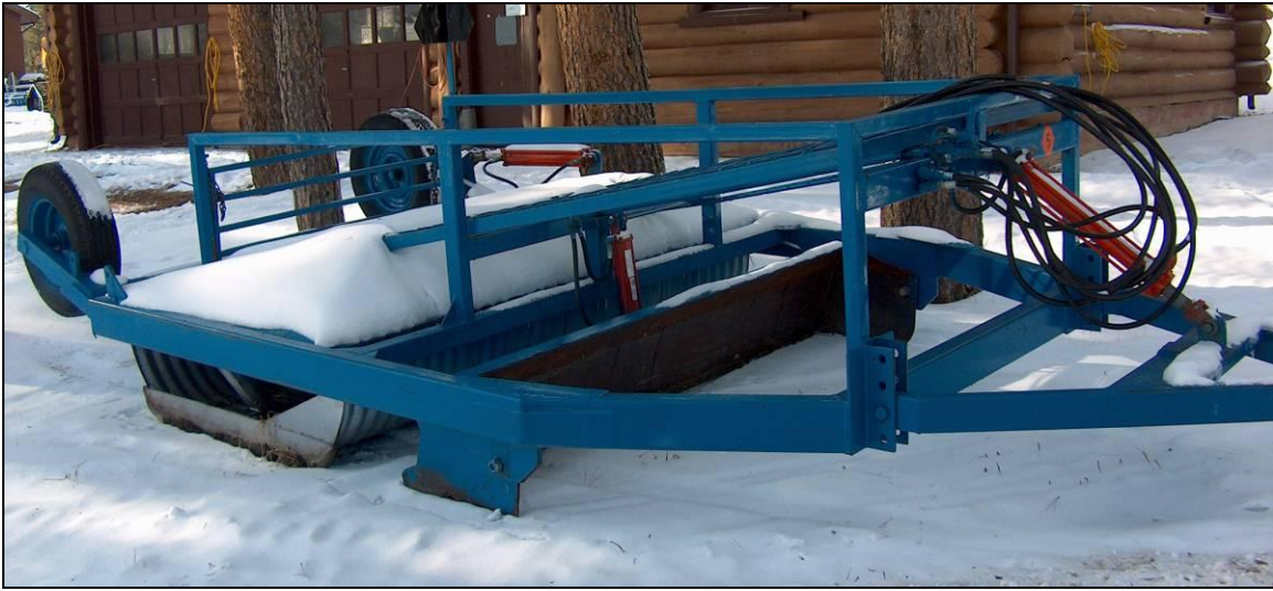
Photo 2.18 Typical single blade drag
