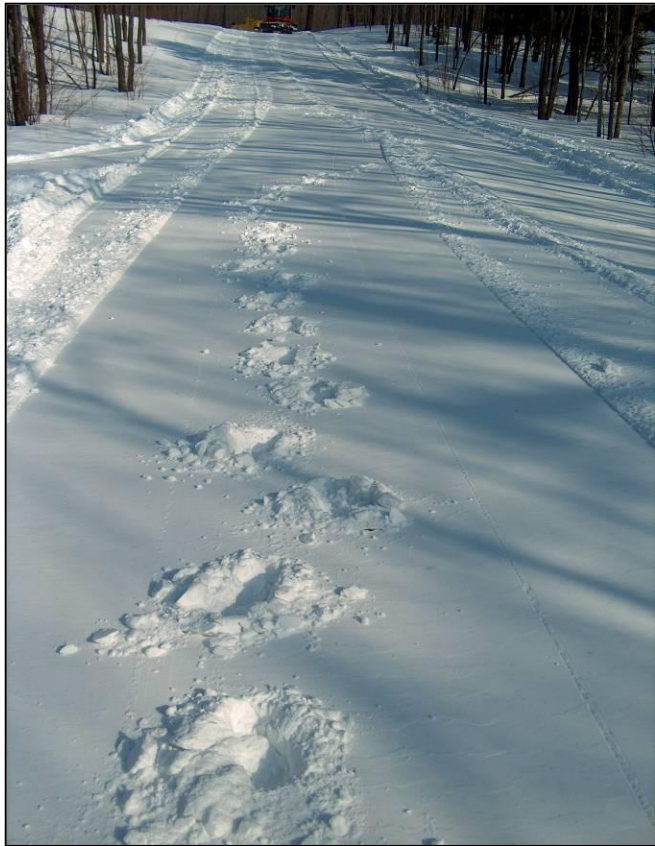
Photo 1.9 Example of a “boot test” that indicates a soft trail
