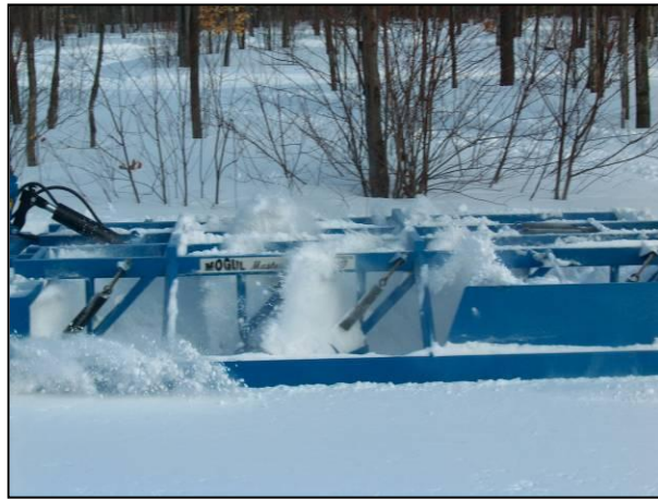
Photo 4.5 Keep processed snow inside the drag!
