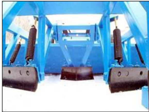
Photo 2.5 Spring tripping blades
