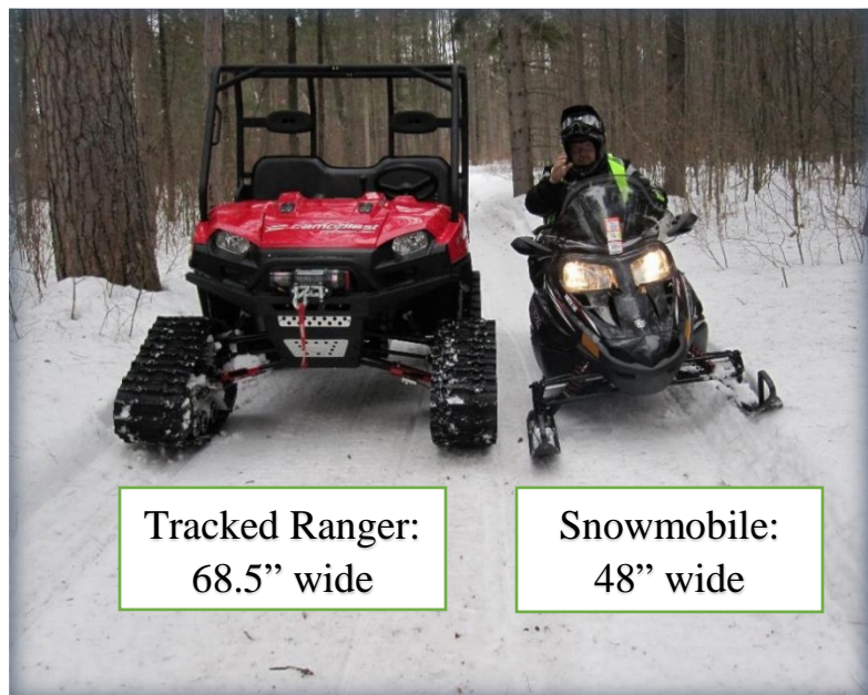
Photo 8: Example tracked UTV width versus snowmobile width
