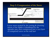
The third step involves the loose snow created by cutting and then churning through the drag's blades being distributed and compressed under the spreader pan. Every time a multi-blade drag works the trail (and has snow being processed through the blades) the trail's depth is increased by a new layer of compacted snow. If snow is all balled up or plugged in front of the spreader pan, the snow will not flow evenly beneath the rear pan — resulting in an uneven or pitted trail surface.
