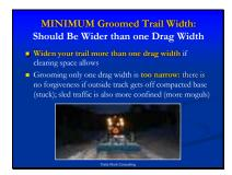
If clearing space allows, the groomed trail should always be maintained wider than only one drag width since there is no 'forgiveness' if the outside track gets off the compacted trail base, particularly when the uncompacted snow beside the trail is deep. Grooming only one drag width wide is generally too narrow since it keeps snowmobile traffic more confined, resulting in more moguls and less enjoyable riding conditions.
