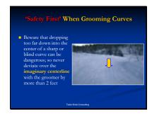
Always think 'Safety First' when grooming through curves. Beware that dropping too far down into the center of a sharp or blind curve can be very dangerous; never deviate over the imaginary centerline (yellow arrow) of the trail with the groomer by more than a couple of feet to ensure any potential on-coming traffic has a place to go.
