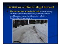
There can potentially be four conditions that limit the groomer operator's ability to effectively remove the entire profile of a mogul. Number one is if there are bare spots in the trail, don't cut deep or try to remove the entire mogul mound since it could damage equipment and also destroy whatever hardened trail base there is. In this case raise the drag's cutting height, perhaps to the point where you're just 'panning' or you may even need to put the wheels down until conditions improve.
